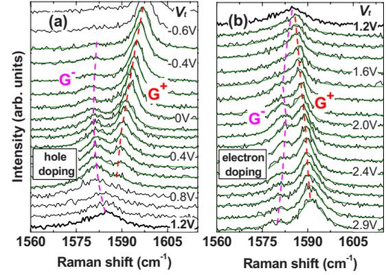
FIG. 3. (Color online) Room-temperature Raman spectra of bilayer graphene biased with the polymer-electrolyte top gate. (a) is for hole doping and (b) is for electron doping.  $V_t = 1.2$  V is the approximate charge neutral position. The smooth overlapping curves are fits with the coupled-mode theory [Eq. (1)] using the parameters in Figs. 4(d)–4(f). Other spectra are fitted with a single Lorentzian (not shown). The dashed lines indicate the peak evolution of the  $G^+$  and  $G^-$  modes.
